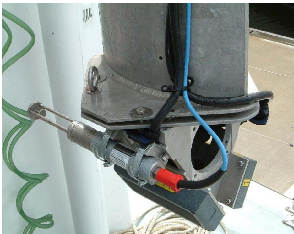
(Figure 4 – SWATHplus-H installed on the hull of the boat)
